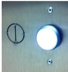
Power Light Illuminated
